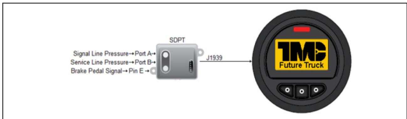
**Figure 1: Prototype of the Proposed Alert Gauge**
