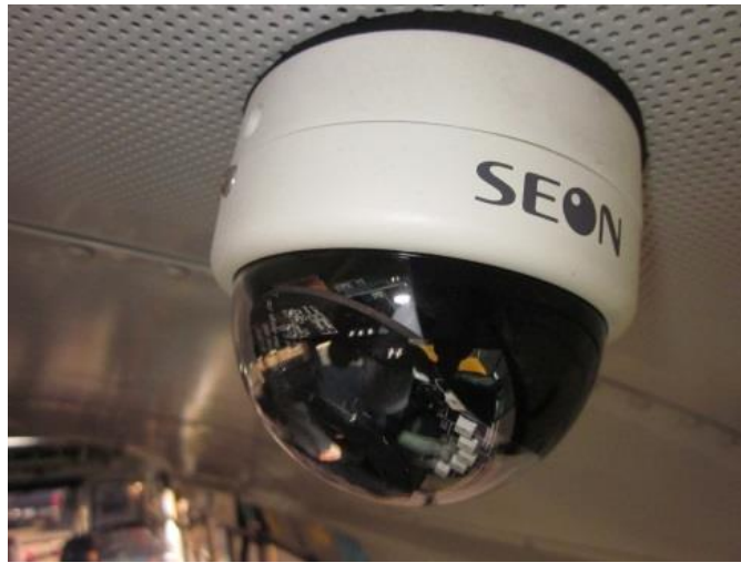
Figure 6. Seon Design interior roof-mounted camera lens in Port St. Lucie school bus.
