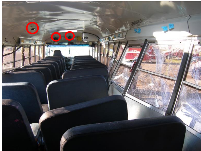
Figure 7. Interior of Port St. Lucie school bus, postcrash, showing locations of three Seon Design interior roof-mounted cameras (circled in red).
